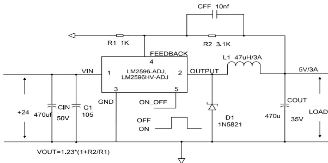
Notes: The circuit and parameters mentioned above are for reference only, and please set the parameters for actual application circuit based on sufficient actual measurement.
